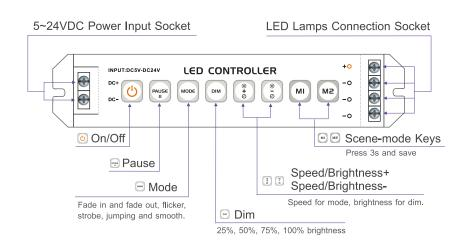
\* Press PAUSE in 3 seconds, the buzzer can be on or off,
